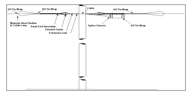
Figure 6 – Cable Storage Loop Using Tie Wraps
