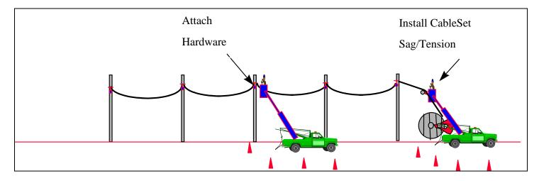
Figure 6 Moving Reel Method
