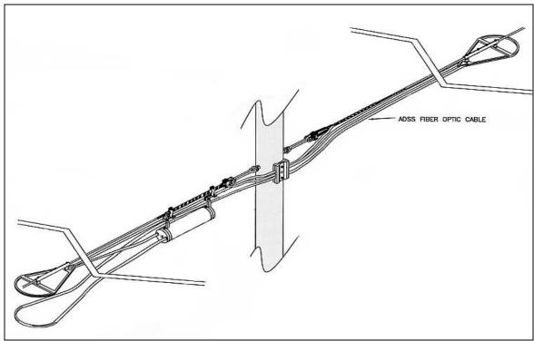
Figure 7 – Cable Storage Using Dulmison Opti Loop
