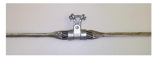
Figure 4 - Intermediate Suspension Attachments – used between dead ends for span lengths up to 600 feet and for line angles up to 20° due to changes in elevation or direction.
