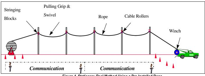
Figure 4 Stationary Reel Method Using a Pre-Installed Rope
