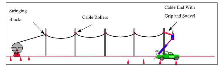
Figure 7 Stationary Reel Method Pulling Cable
